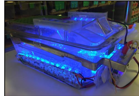
Sterile cages with blue light ( \lambda 450nm)
